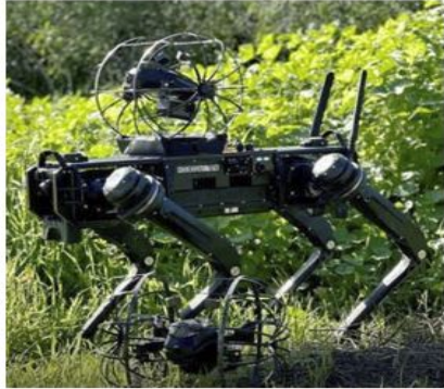
The US-made Vision 60, a dog-shaped walking robot. Another robot, Israeli-made, called the Rooster, is installed on the robot's back, creating a kind of ground robot and drone. (photo)
